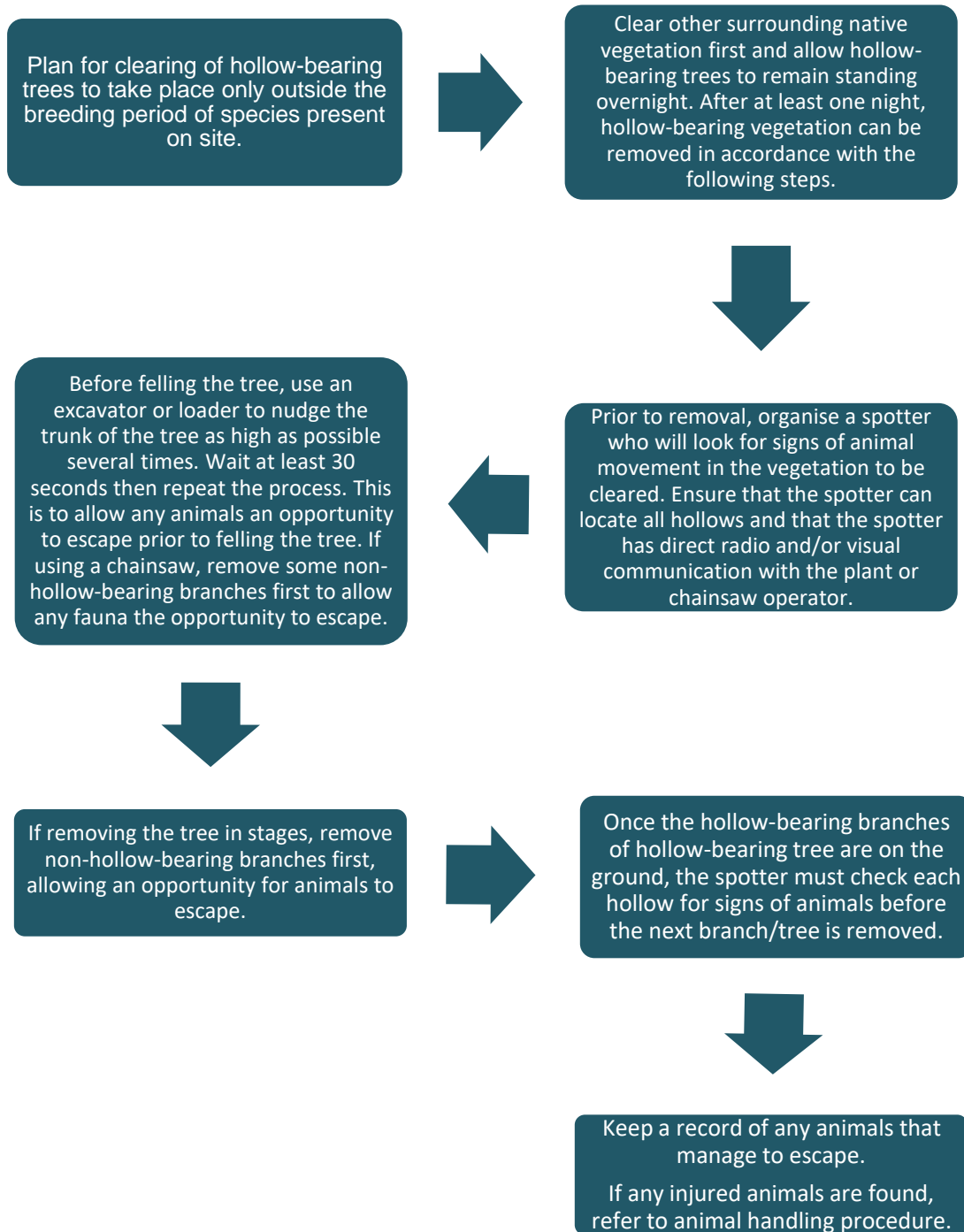
Figure 7-5 Hollow bearing tree removal procedure
