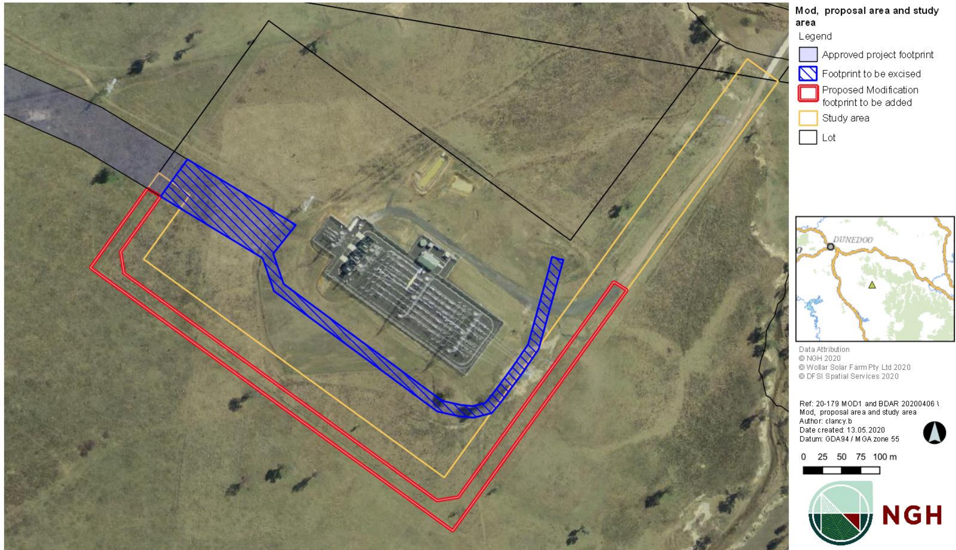
Figure 1-3 Areas to be excised (in blue) and added (in red) for the modification
